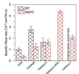
**Figure 8. Specific wear rate of the coatings**
