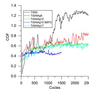
**Figure 7. Coefficient of friction of the films tested at 600°C**
