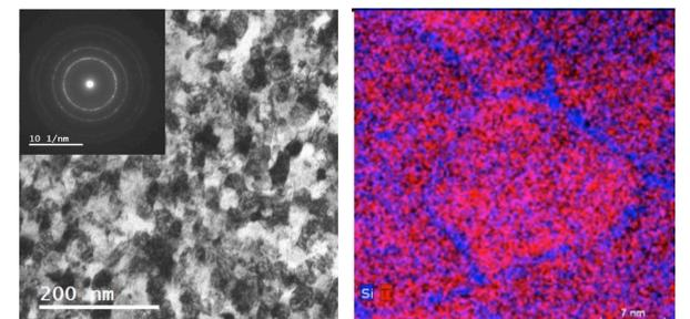
**Figure 5. Structure of the TiSiN reference film**
