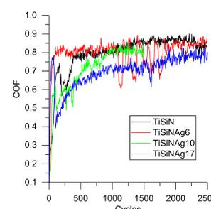
**Figure 6. Coefficient of friction of the films tested at room temperature**
