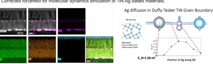
Elemental STEM/EDS maps the distribution of a TiN/TiN(Ag)/TiN stack layer annealed at 800 °C for two hours showing the diffusion of Ag and the path on TiN layers.
