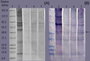
**Fig.3** SDS-PAGE (A) and WB (B) of *Pg* extract antigens before and after encapsulation into the PLGA-CS nanocarrier. Lanes: (1) MW marker (2) native *Pg* extract antigens; *Pg* extract antigens from PLGA-CS NPs prepared with antigen amounts of (3) 500, (4) 750, (5) 1000  $\mu$ g. Kgp gingipain: 56 kDa.
